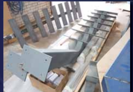
Stairs all etch primed and packaged ready to ship locally or interstate.
