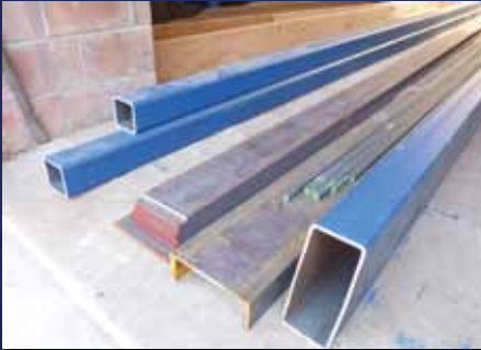
Beams come in options: RHS 200mm x 100mm x 6m or 200mm x 150mm x 6m
