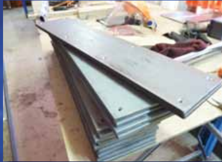
Plates cut to size & drilled
