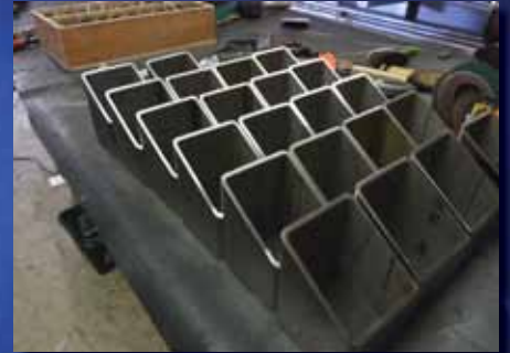
Stumps cut to angle & length
